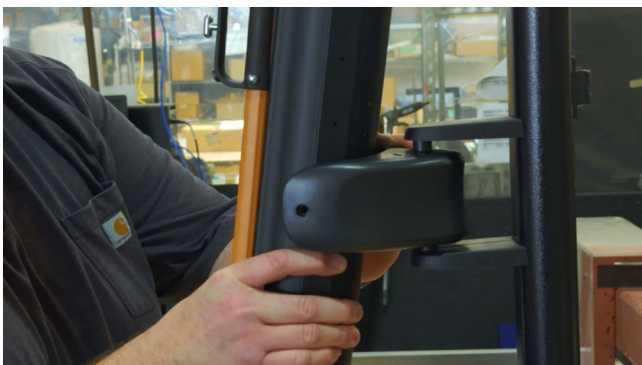
5 Position the housing onto the bracket.
